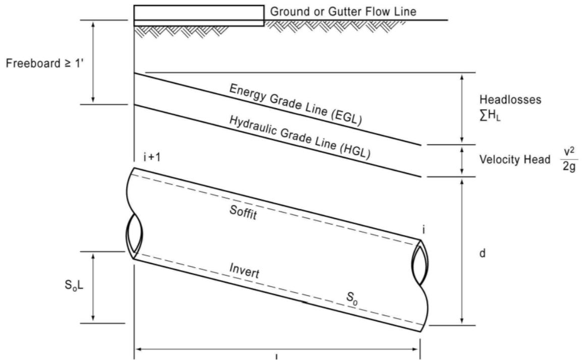
**Figure 2-2** Definition Sketch for Storm Drain Hydraulic Calculations
