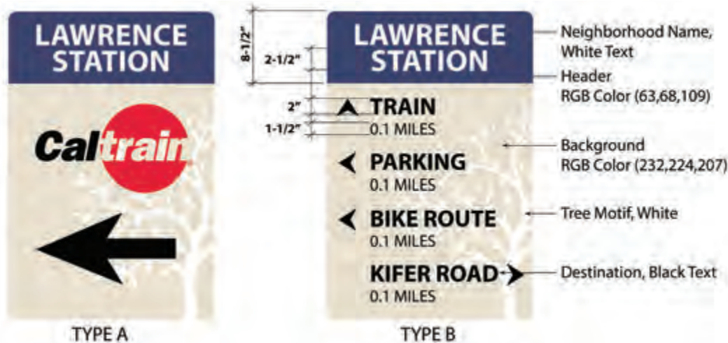
Figure 3-22. Directional Sign Enlargement
