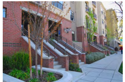
The first floor of residential units should transition from the street with raised stoops or steps.
